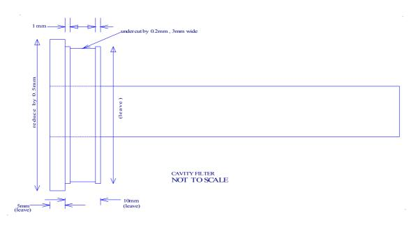
With a 10mm overlap, and four screws, the cavity length had a possible variation of several millimetres as to exactly where the outer short circuit was located, so the set frequency of the cavities could wander by about 100 times the precision we needed to maintain. Within our club we had some members with experience in this technology, so a suggestion was made to machine the top plates as shown.
