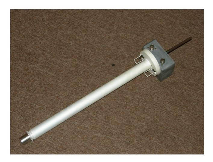
Replacing that surface layer with silver plating seemed to be the answer, but great care is needed here. Most firms that do silver plating do "decorative" silver, for spoons, jewelery etc. and this process uses what they call "brighteners", that is about 5% of the plating is nickel. The effect of this on RF circuits is to ruin the performance.
