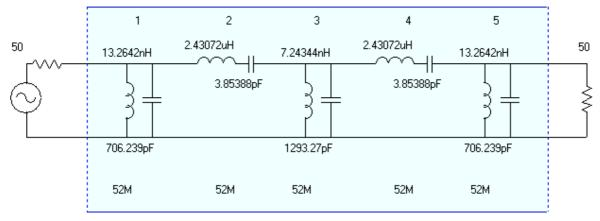
Next click on Analysis and set Start Frequency say 20Mhz, Stop Frequency 100Mhz, Loss Bottom db -120, and the defaults should be ok for the rest. It is most important that you use the upper case "M" after any frequency, otherwise you get really strange results. Then you can click on Plot, to see a range of things, I generally click on the 6<sup>th</sup> down from the top of the 12 choices on the left. You then get the frequency response in red and the VSWR in blue, see page 4.
