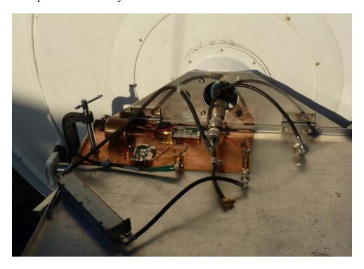
Fig 3 The feed to the 1.2 m dish showing the low noise preamplifier.
