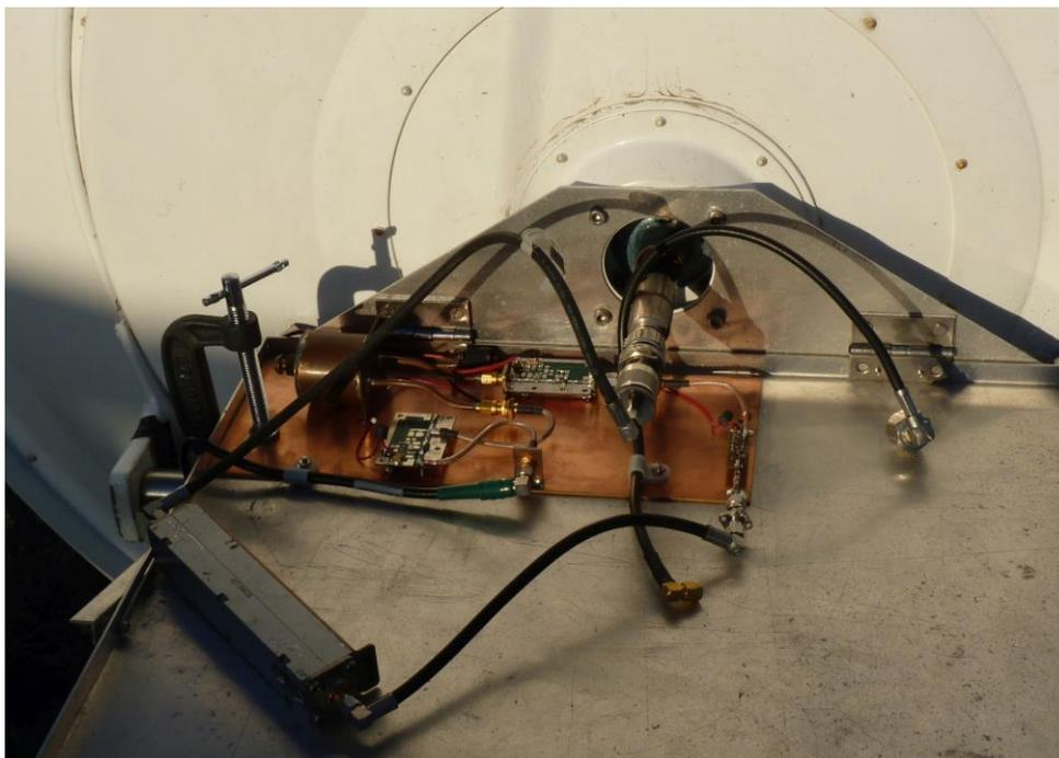
**Fig 3 The feed to the 1.2 m dish showing the low noise preamplifier.**
