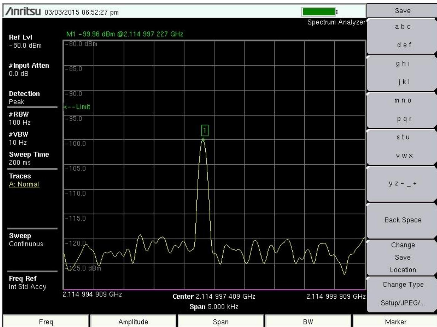
Fig 2 Spectrum Analyser EME Signal Detection
