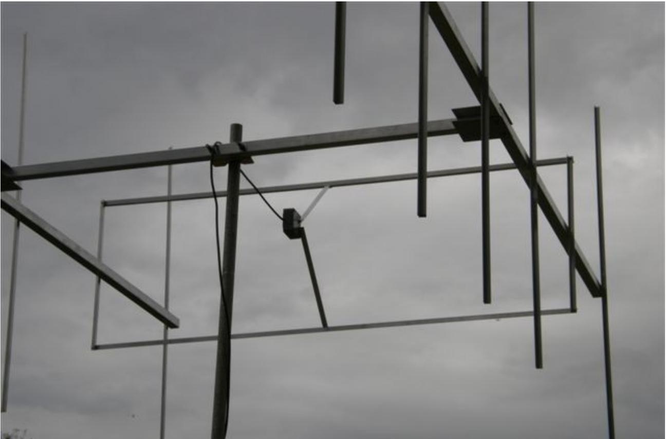
Here is a close up of the driven element, which is the actual skeleton slot. It is  $5/8$  wavelength in the direction perpendicular to the radiation polarization, and  $5/16$  wavelength for the driven element part of each yagi. This sets the spacing between the two yagis at  $5/8$  wavelength too.
