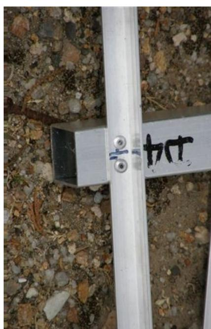
The driven element can be pop-riveted or screwed together, but I wanted to be able to pack the aerial onto a car roof rack, to set it up on field days, so I assembled it with M3 stainless steel nuts & bolts.
