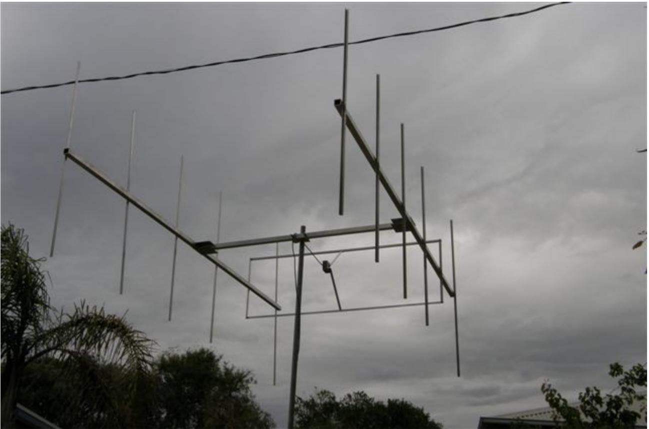
The skeleton slot was developed in the UK for TV use soon after WW2. Someone had worked with slot aerials on aircraft, and the use of a half wave vertical slot in a very large piece of sheet metal, results in radiation very much the same as a horizontal dipole. They then set out to find out how much you could reduce the metal around the slot, and have it still radiate.
