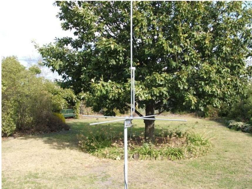
An alternate mounting method which includes ground plane radials.
