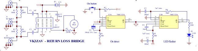
I find that flat batteries are a constant nuisance, because its too easy to leave it switched on, so I've included a timer that gives about 10 minutes operation after pressing the start button.
