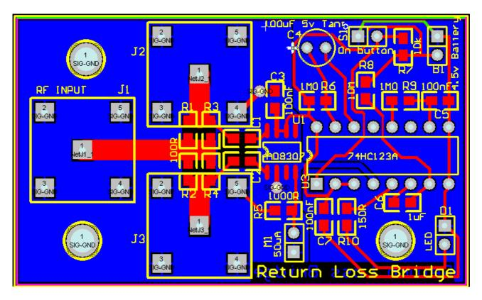
To use as a milli-voltmeter, short-circuit J1 and feed the signal into J2 or J3. The input is terminated in 50  $\Omega$ .
