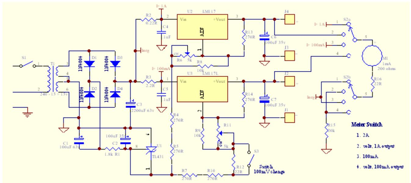
The circuit starts with a transformer, in this case I've used one with two 15v secondary windings, but up other voltages can be used. The diodes D3 & D4 rectify the transformer volts, and C3 filters the ripple. This then feeds into the two regulator chips, an LM317L (TO-92) low current, 100mA output, and an LM317 (TO-220) for the 1A output. Each regulator is current metered on its input via R2 & R3, and each output is independently adjustable via the pots R6 and R8.
